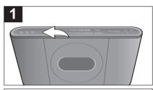
Slide the CD DOOR OPEN switch to the right and the CD door will open. Gently insert a CD onto the spindle (label side facing forward) until it clicks. Close the CD door.
